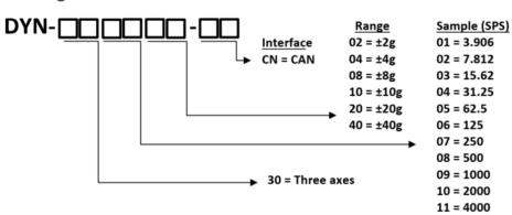
**Example:** DYN-301140-CN: Triaxial, 4000 SPS, ±40 g, Capacitive Accelerometer with CAN Interface.
