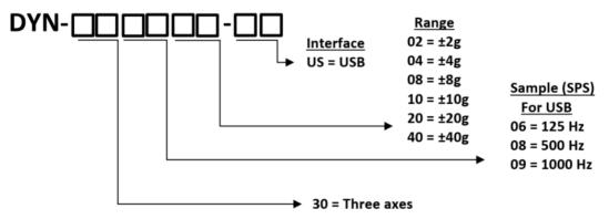
Example: DYN-300840-US: Triaxial, 500 SPS, ±40 g, Capacitive Accelerometer with USB Interface.
