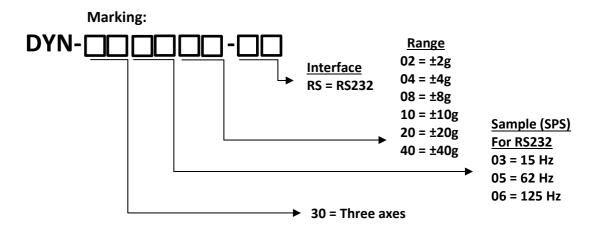
**Example:** DYN-300640-RS: Triaxial, 125 SPS, ±40 g, Capacitive Accelerometer with RS232 Interface.
